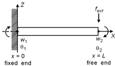
Fig. 3 Flexible cantilever beam element
