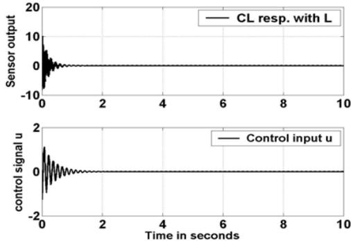
Fig. 8 CL impulse response with FOS feedback gain  $L$  (sensor output  $y$ ) and control input  $u$ , beam divided into 4 finite elements, PZT placed at fixed end
