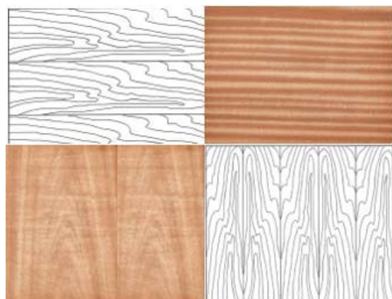
Fig. 11 The combination of horizontal placed quarter sliced slip matching with vertical placed flat sliced book matching panels creates a rich decorated interior design [11]
