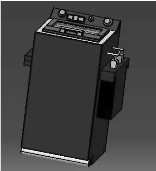
Fig. 3 The conceptual design of the main physical body of the variable volume and the variable spinning speed washing machine
