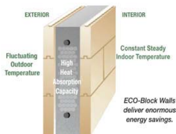
Fig. 11: Structure of Eco-Block Wall [18]
