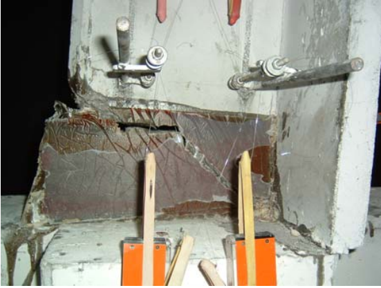
Fig. 2 A view of corbel and bottom side of the beam at the CP1R specimen after experiment
