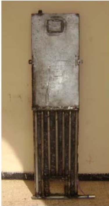
Fig. 2 Absorber made by tubes and galvanized tank
