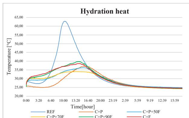
Fig. 4 Evaluation of hydration temperatures
