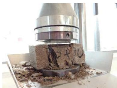
Fig. 5 Testing compressive strength
