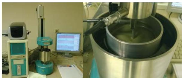
Fig. 2 Rotary viscometer ViskomatNT
