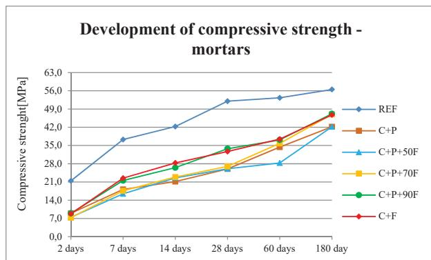
Fig. 6 Results of compressive strength testing
