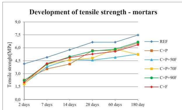
Fig. 7 Result of tensile strength after bending
