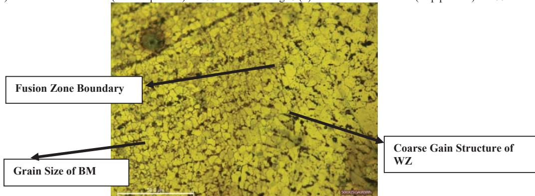
Fig. 6 (c) Microstructure of HAZ at 500X
