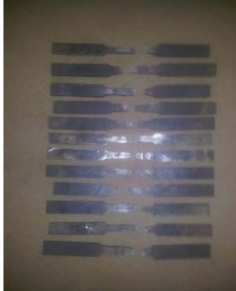
Fig. 2 (a) Fractured tensile test samples of Schemes 1 &amp; 2
