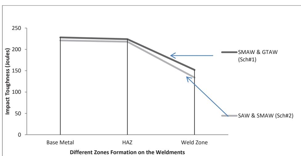
Fig. 3 Impact Toughness of Hybrid welding Schemes 1 &amp; 2
