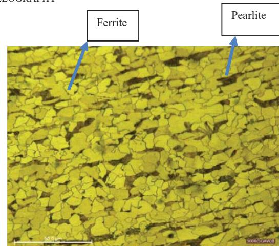
Fig. 5 (b) Microstructure of Base metal 500 X
