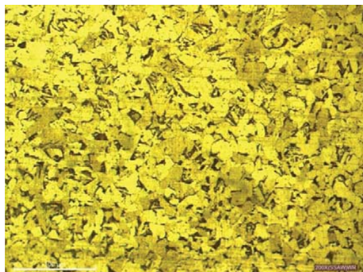
Fig. 7 (a) Microstructure of WZ (Root portion) at 200X
