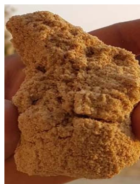
Fig. 9 Sample with a good cementation after treatment from third trail
