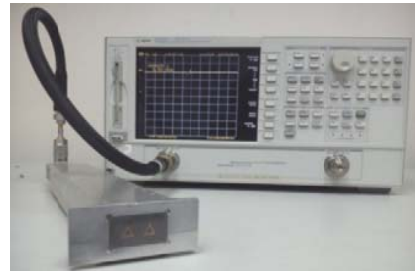
Fig. 5 Scattering parameters measurements setup
