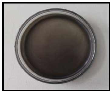
Fig. 1 Sample of PVDF/OG obtained by the conventional casting technique (slow evaporation at 60°C)
