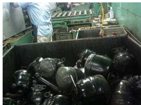
Fig. 6 Compressors Divided from Waste Home Appliances
