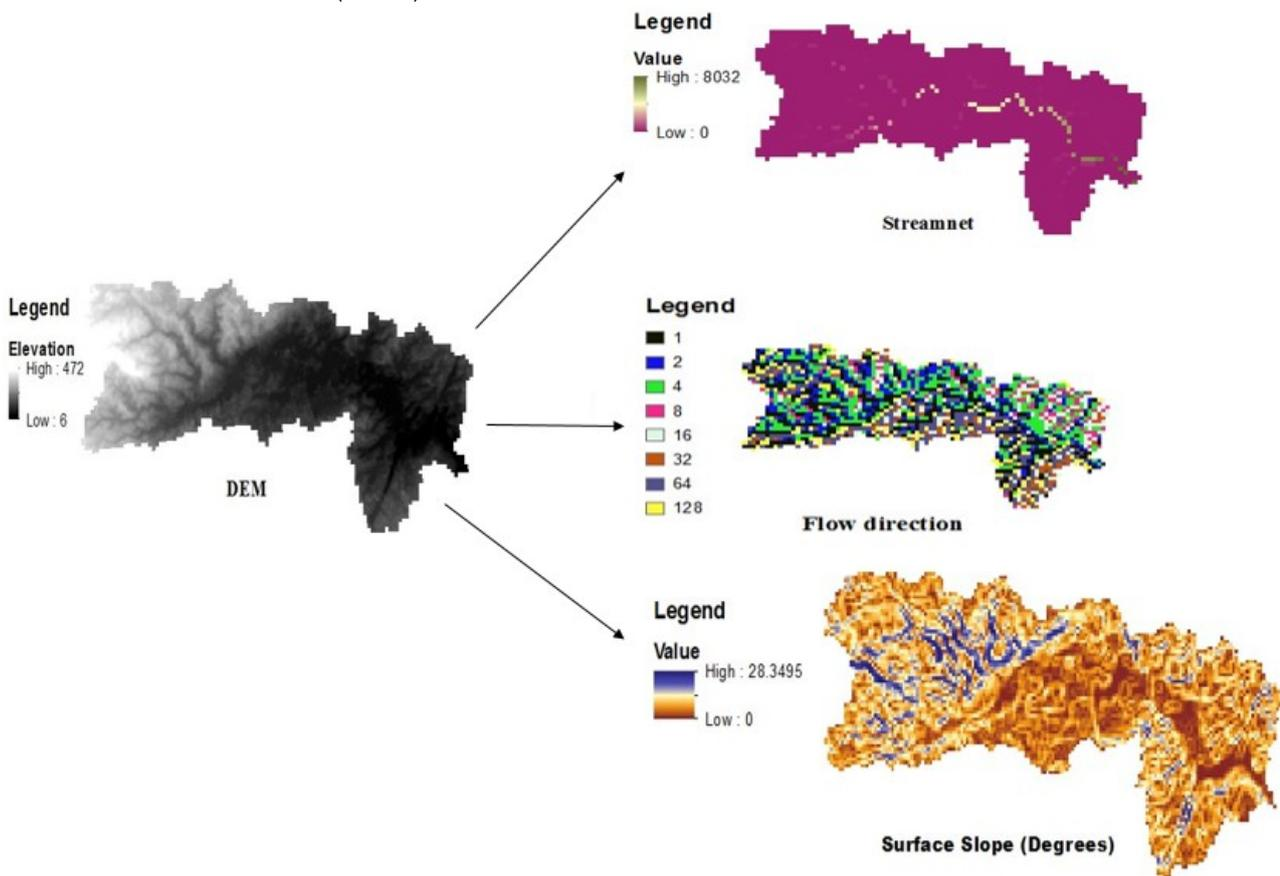
Fig. 4 Topographic data maps for PyTOPKAPI model input
