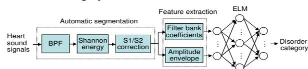
Fig. 1 The ELM-based heart sound classification system.
