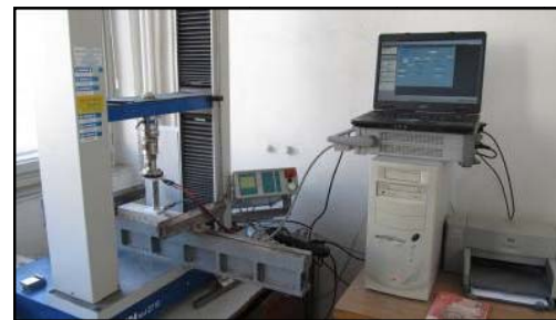
Fig. 2 Evaluation of electrical properties under loading
