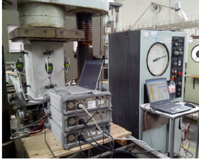
Fig. 5 The model column in the hydraulic press machine connected to the equipment monitoring changes in deformation and impedance
