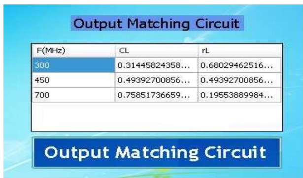
Fig.10 The output constant gain circles radius and center.
