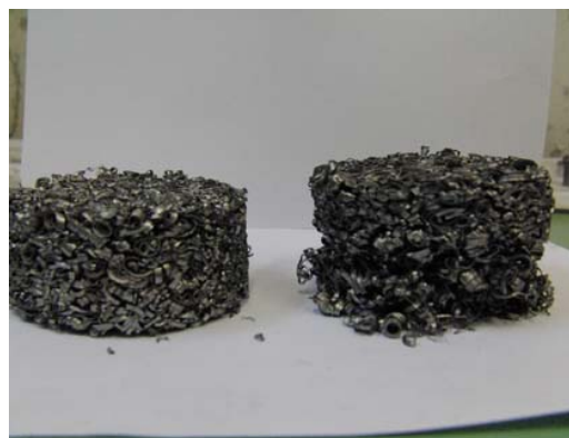
Fig. 3 Briquettes from Armco iron chips with 80 mm diameter: left – after one impact; right – after two impacts
