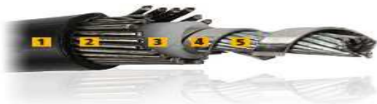
Fig. 4 Construction of Bowden cable 1) plastic sheathing 2) outer sheathing made of spring steel wire 3) Teflon guide sleeve 4) spiral wire 5) inner core made of spring steel wire [14]
