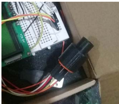
Fig. 3 Mouthpiece with MQ 138 sensor
