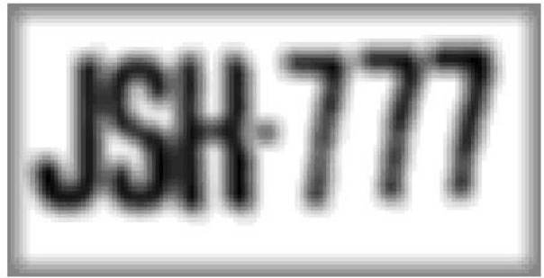
Fig. 13: Blurred image of a number plate is generated by linear image degradation model.
