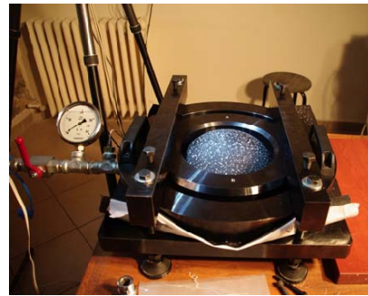
Fig. 3 Pneumatic Bulge Test Assembly
