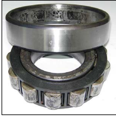
Fig. 12 The bearing after removal. Note the marks in the rollers and the outer race
