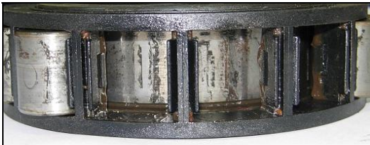
Fig. 15 The defects (dark marks) in the inner race of the bearing
