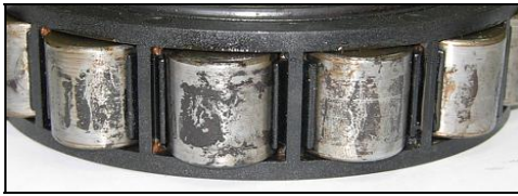
Fig. 13 The defects (dark marks) in the rolling elements of the bearing
