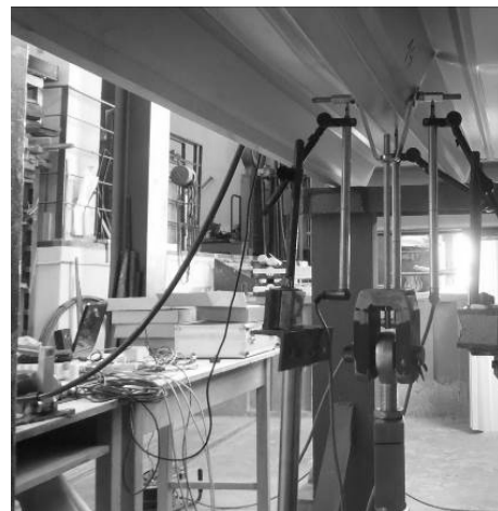
Fig. 4 Measuring instruments to vertical deflection
