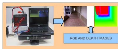
Fig. 5. Robot Sensor Data Capturing Platform
