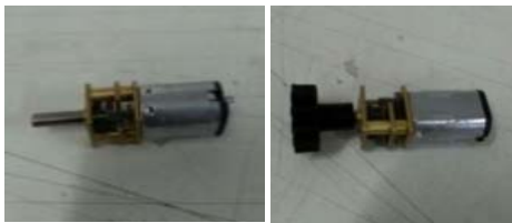
Fig. 6 DC Motor and Gear Motor Mounted to Shaft
