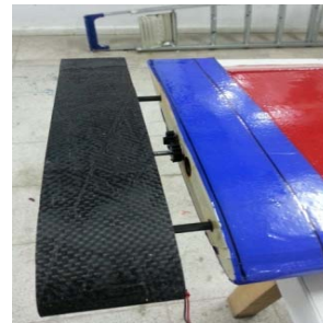
Fig. 9 Montage of the Expanding Parts of the Wing
