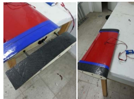
Fig. 11 Morphing Wing Tip Assembly
