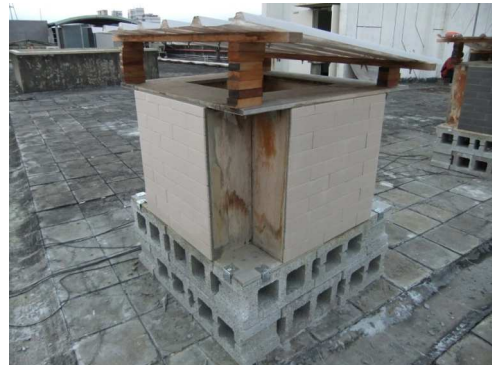
Fig. 5 Experimental group consisting of tiled exterior walls
