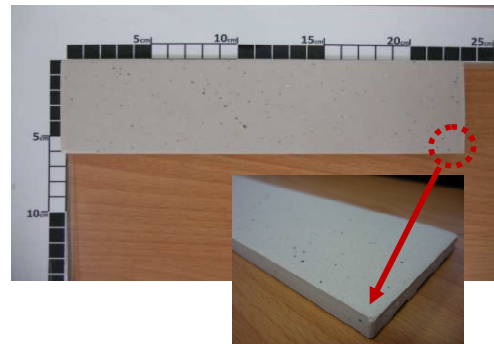
Fig. 6 Exterior wall tiles used in the experimental group
