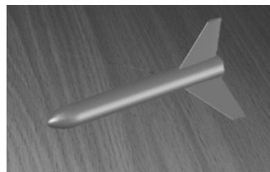
Fig. 3 Wing-body-tail configuration
