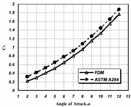
Fig. 8 Comparison of normal force coefficient at Mach 0.5
