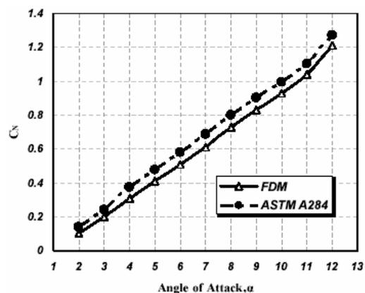
Fig. 5 Comparison of normal force coefficient at Mach 0.3
