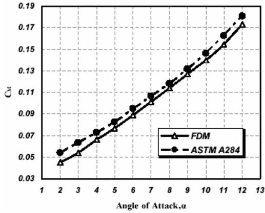
Fig. 6 Comparison of pitching moment coefficient at Mach 0.3
