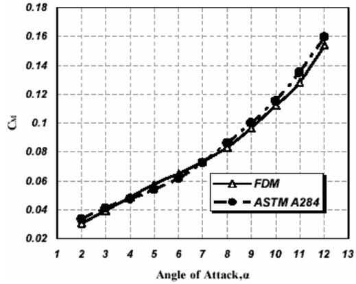
Fig. 9 Comparison of pitching moment coefficient at Mach 0.5
