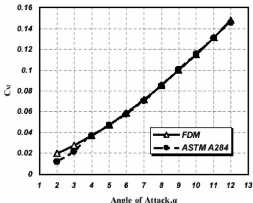
Fig. 12 Comparison of pitching moment coefficient at Mach 0.75
