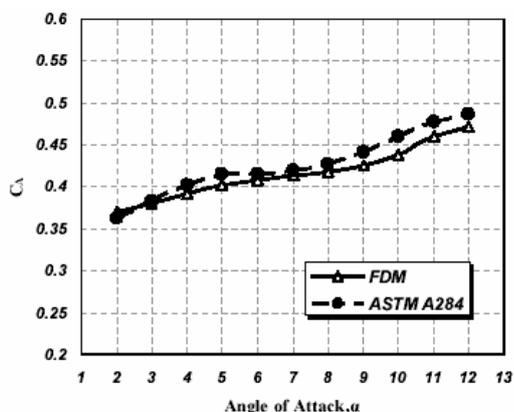
Fig. 13 Comparison of total axial force at Mach 0.75
