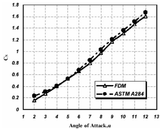
Fig. 11 Comparison of normal force coefficient at Mach 0.75
