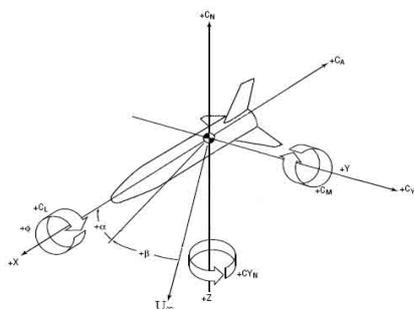
Fig. 4 Wing-body aerodynamic axis system
