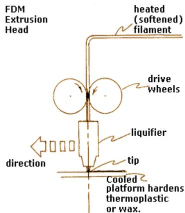
Fig. 1 Fused Deposition Modeling (FDM) rapid prototyping process
