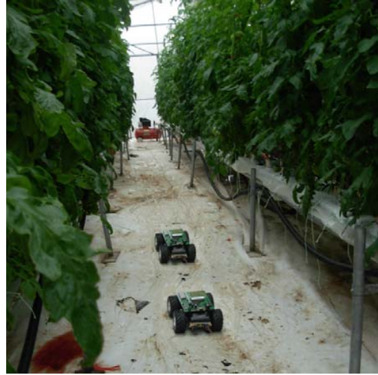
Fig. 6. UGV robot formation in a greenhouse corridor.
