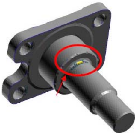
Fig. 1 Critical stress location
