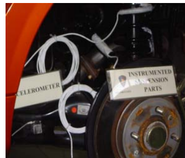
Fig. 2 Instrumented suspension system
