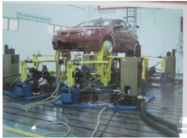
Fig. 3 MTS 320 multi-axial spindle coupled road simulator
