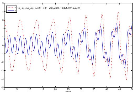
Fig. 1. Plots of  $x = x_0 + x_1$  and  $y = y_0 + y_1$  for  $[\omega_1, \omega_2, \tau, \alpha_1, \alpha_2, \varepsilon, x(0), \dot{x}(0), y(0), \dot{y}(0)] = [1, 3, 5, 1, 1, 0.1, 3, 0, 1, 0]$ .
