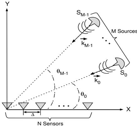
Fig. 2. Uniform Linear Array in 2-D geometry.
