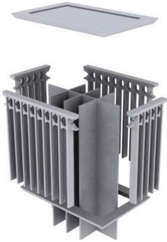
Fig. 4. 3D model of a Wind catcher with equal canals
