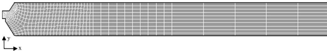
Fig. 4 Plate 2D finite element mesh
