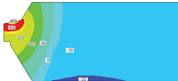
(a) Residual stress contour of critical points
