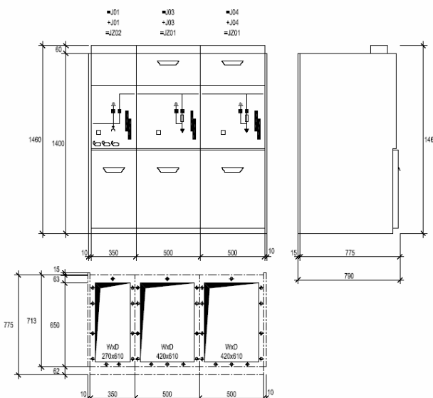
Fig. 3 Sketch of medium voltage fields
