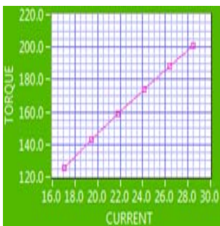
Fig. 4 Torque vs current characteristics of dc motor
