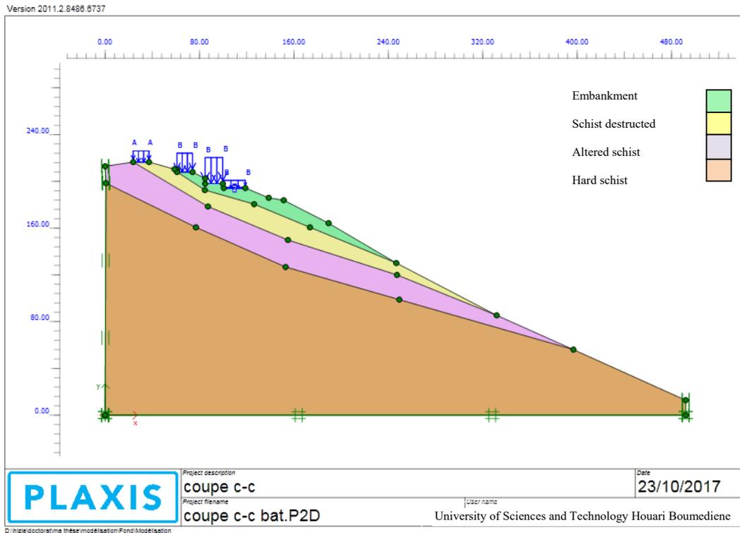
Fig. 2 C-C in middle of landslide of AEH (view Plaxis model)
