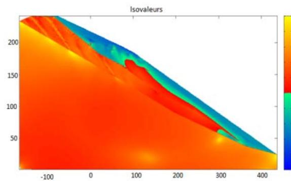
Fig. 5 Second order work of section C-C
