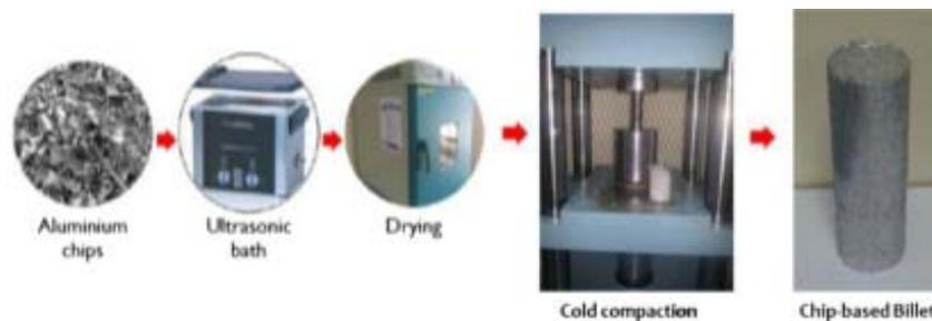
Fig. 2 Preprocessing of chips before consolidation
