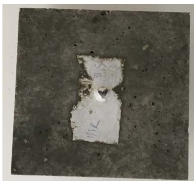
Fig. 5 Cube specimens before compressive strength test
