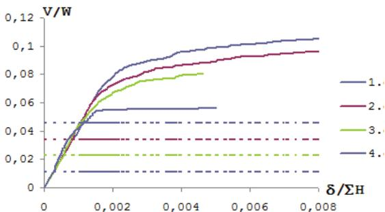
Fig. 9 Load-Displacement curves for 6-story buildings for Z1
