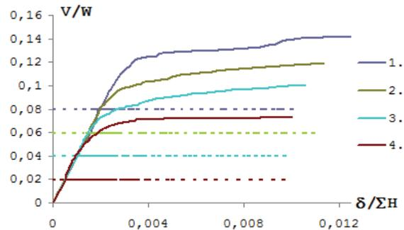
Fig. 11. Load-Displacement Curves for 6-story buildings for Z3
