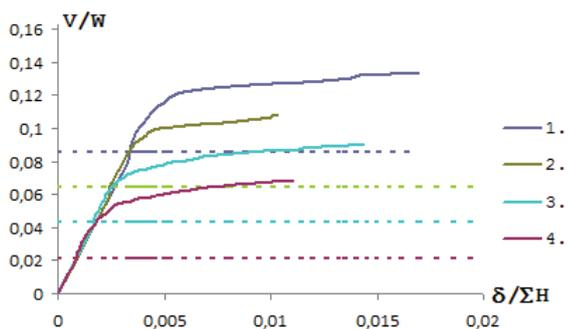
Fig. 16 Load-Displacement curves for 8-story buildings for Z4
