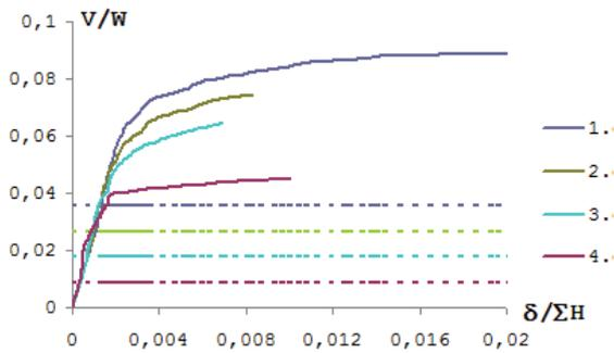
Fig. 13 Load-Displacement curves for 8-story buildings for Z1
