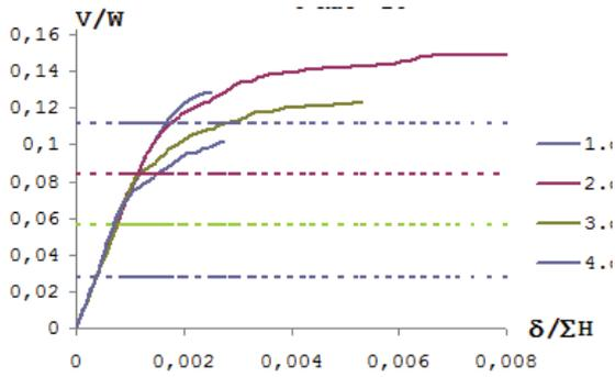
Fig. 8 Load-Displacement Curves for 4-story buildings for Z4
