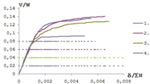
Fig. 5 Load-Displacement curves for 4-story buildings for Z1
