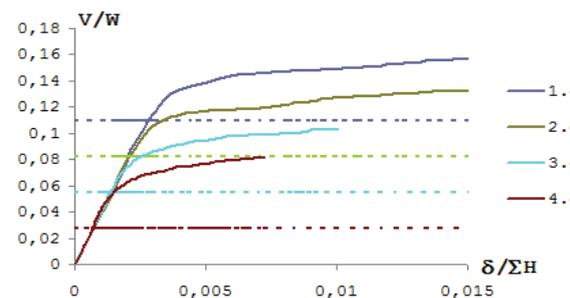
Fig. 12 Load-Displacement curves for 6-story buildings for Z4
