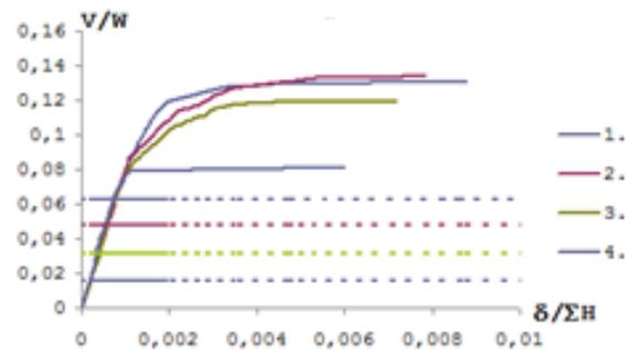
Fig. 6 Load-Displacement curves for 4-story buildings for Z2
