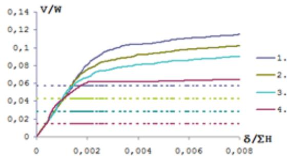
Fig. 10 Load-Displacement curves for 6-story buildings for Z2
