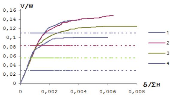
Fig. 7 Load-Displacement curves for 4-story buildings for Z3
