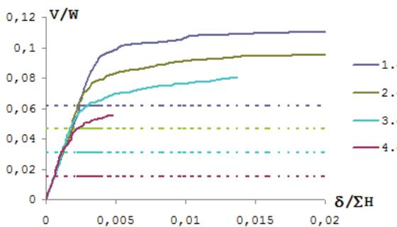
Fig. 15 Load-Displacement curves for 8-story buildings for Z3
