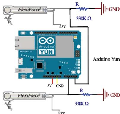
Fig. 5 The main circuit of the system
