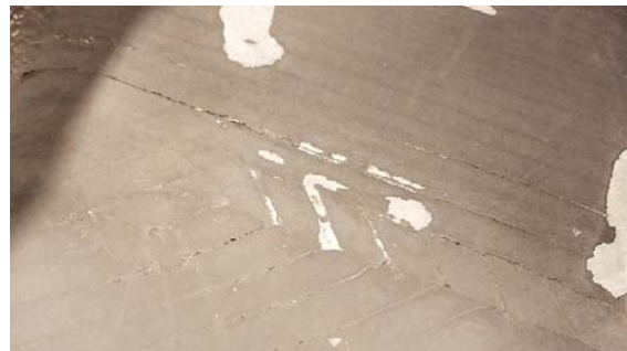
Fig. 11 Cracking defects of the mold surface
