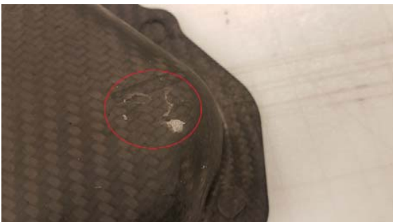
Fig. 15 Carbon fiber valve cover defects
