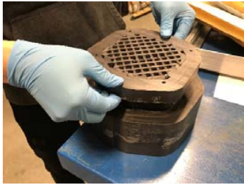
Fig. 7 Completed compression mold assembly
