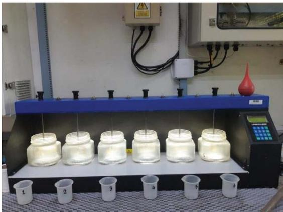
Fig. 2 Jar test equipment
