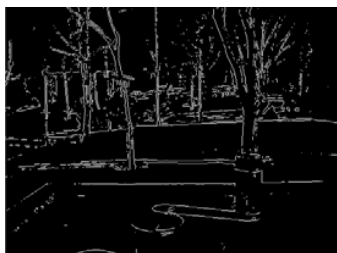
Fig. 5. Edge detection by canny operator (only Phase 2)
