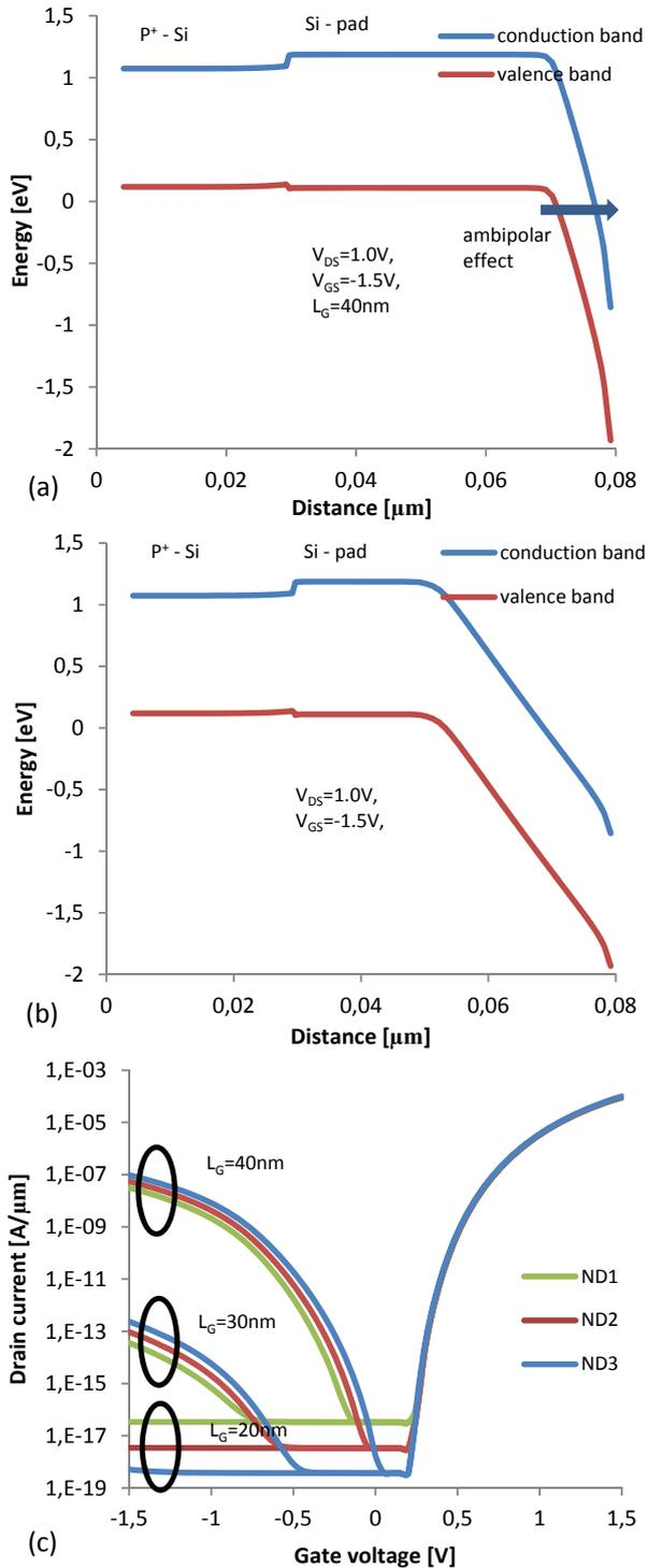
Fig. 4 (a) Band profile of DGPNTFET for gate length ( $L_G$ ) = 40nm at  $V_{DS}=1\text{V}$ ,  $V_{GS}=-1.5\text{V}$  (b) Band profile of DGPNTFET for  $L_G = 20\text{nm}$  at  $V_{DS}=1\text{V}$ ,  $V_{GS}=-1.5\text{V}$ . (c) Transfer characteristics of DGPNTFET for different gate length ( $L_G$ ) (where  $N_{D1}=1\times 10^{15}\text{ cm}^{-3}$ ,  $N_{D2}=1\times 10^{16}\text{ cm}^{-3}$ ,  $N_{D3}=1\times 10^{17}\text{ cm}^{-3}$ )
