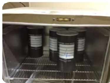
Fig. 7 Storage of mortar bars for AMBT test
