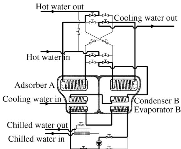
Fig. 8 The mass recovery-like process of [27]
