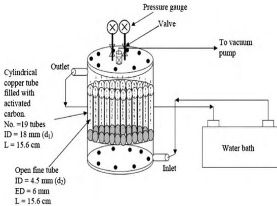
Fig. 7 The adsorption system used in [26]
