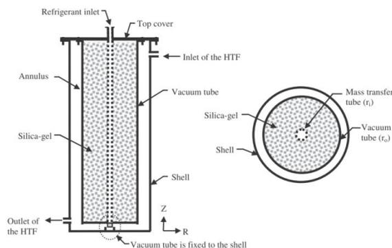
Fig. 3 Schematic view of the cylindrical adsorbent bed [15]
