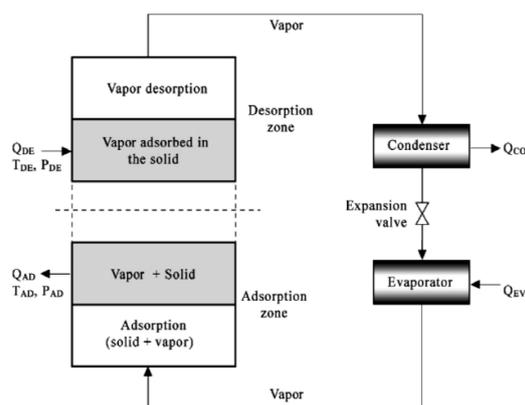
Fig. 1 Schematic diagram of the adsorption refrigeration cycle [2]
