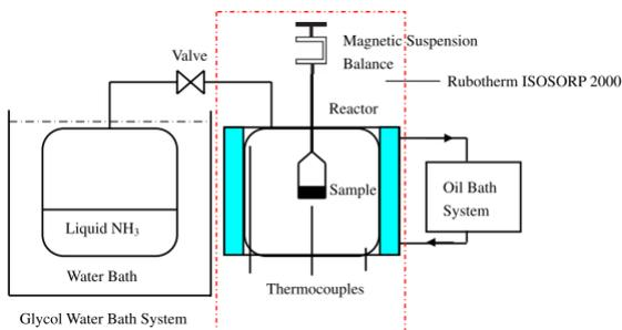
Fig. 14 Schematic diagram of porosity test rig [33]
