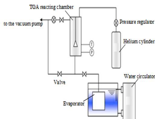
Fig. 12 Schematic diagram of the experimental set up [31]
