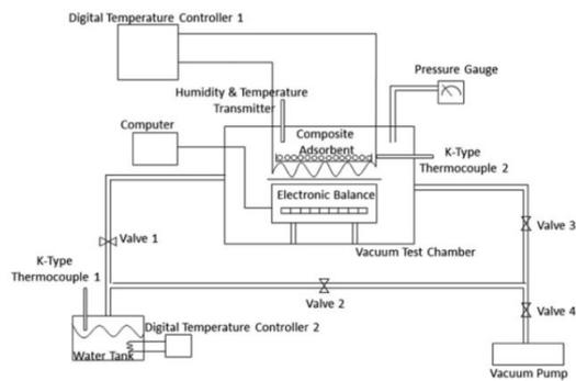
Fig. 4 Schematic diagram of the adsorption test unit [18]
