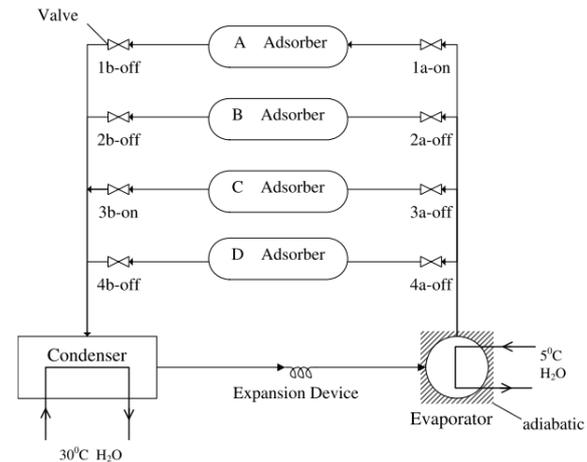
Fig. 10 The multi-bed adsorption heat pump of [29]
