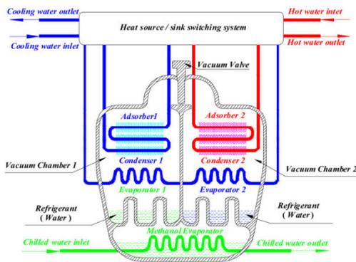
Fig. 9 Schematic diagram of the adsorption chiller of [28]
