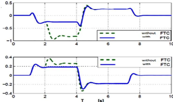
Fig. 6 The simulation of the residual  $r_1$  and  $r_2$  using the FTC approach and without FTC approach
