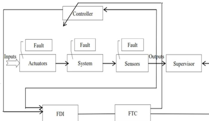
Fig. 1 Process description using the FDI and FTC [9]
