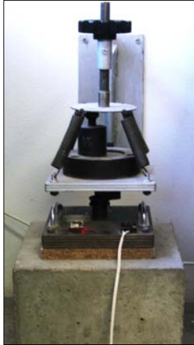
Fig. 3 Measurement of dynamic stiffness
