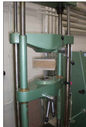
Fig. 2 Measurement of tensile strength
