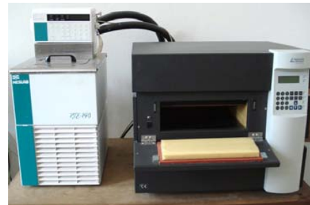
Fig. 1 Apparatus Holometrix 2300 for determination of thermal conductivity
