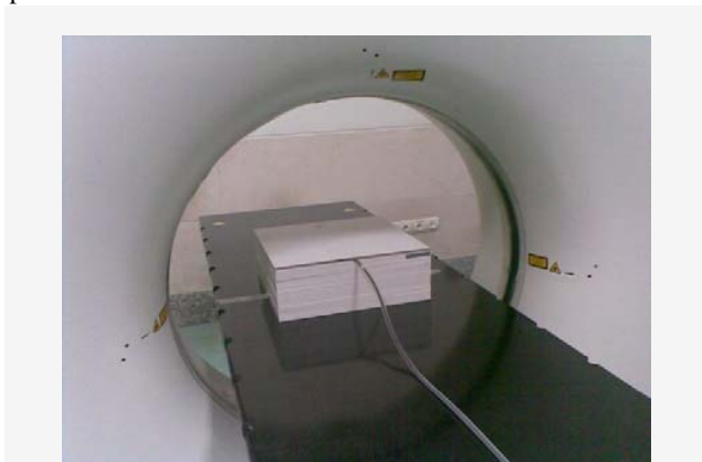
Fig. 1 phantom placed in CT scan device
