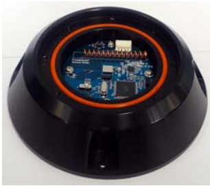
Fig. 2 The sensor node in enclosure (lid not shown)
